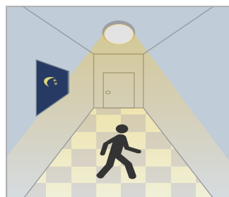
When motion detected, insufficient daylight, light ON.
